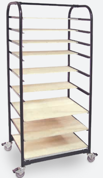
brent® Ware Cart EX Heavy-duty ware cart features top/bottom frame supports that bolt into place and powder-coated frame for durability and improved scratch and corrosion resistance. Side frames are 12-gauge steel with welded shelf supports. Square cross support tubes are 11-gauge steel. 35"W x 24"D x 72¾"H. The 4 heavy-duty, 4" rubber swivel casters roll easily when cart is loaded and can be firmly locked in place when needed. Comes with a set of 12" x 32", ½" thick exterior plywood shelves (shipped in a separate carton). Also includes plastic cover. Ware cart is shipped unassembled in 1 carton. Allow extra delivery time. 🚚 Z08621 — $995.95
