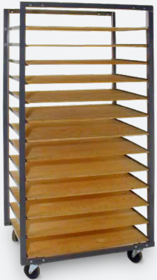
Bailey Ware Trucks Constructed of heavy-duty angle iron, vertical posts, and heavy gauge galvanized rungs. Each rack comes complete with 6" casters. The 13-division rack includes 13 pairs of rungs; the 26-division rack includes 26 pair of rungs that can be bolted in place at any spacing desired. Ideal for dinnerware or tile production. Shelves not included. Assembled dimensions: 34½"W x 24"D x 74¼"H. Assembly required. Allow extra delivery time. 13-Division Rack 🚚 Z15242 — $1,122.65 26-Division Rack 🚚 Z15243 — $1,544.95 Ware Boards. ½" AC plywood. 9719057 Half shelf, 12" x 32" — $22.90 9719058 Full shelf, 24" x 32" — $46.30
