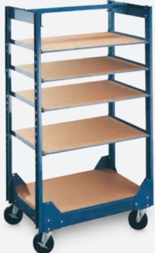
North Star Shelf Truck Fully adjustable, heavy-duty ware truck. Shelves supported at each end by brackets that adjust instantly to any level. Solid steel frame. Full 6" dia. industrial swivel casters (2 with brakes) carry up to 750 lbs. Comes with 5 shelves and 4 pairs of shelf brackets (first shelf goes directly on frame). For storing and transporting clay and kiln furniture as well as ware in progress. 37"W x 24"D x 66"H. Assembly required; shipped in 3 cartons. Allow extra delivery time. 🚚 Z13987 — $1,300.00
