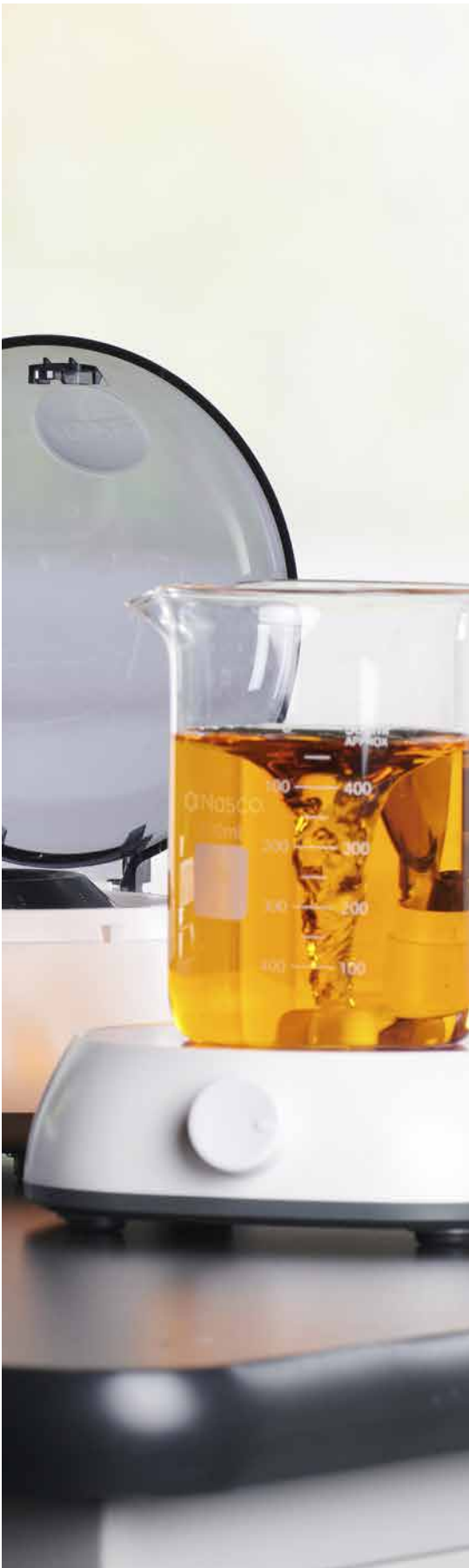
Magnetic Stirrer with Heater Simultaneously stirs and heats liquid. Totally enclosed, cast aluminum heating surface resists chemical spills. Separate dials regulate stirring speed and temperature. Has 1" octagon stir bar with molded-on pivot ring in center, detachable 1' support bar with thermometer/pH probe clamp, and detachable power cord. Stirring capacity: up to 500 ml with a strong vortex. 180 watts. Temperature max.: 480° F (250° C). 120-1600 rpm. 5" x 5" SB48265 110V — $195.00 SB52702 220V — $197.00 7" x 7" SB51127 110V — $260.00 *EXCLUDED FROM DISCOUNTS SB52703 220V — $255.00 *EXCLUDED FROM DISCOUNTS
