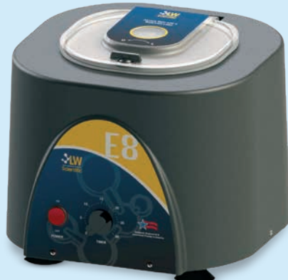
E8 Centrifuges • Accommodates most test tubes from 3-15 ml • Wide stance and suction-cup feet eliminate wobbles, vibrations, and slipping • Brushless motor is virtually maintenance-free • Auto switching between 110V and 220V • Includes 8-place tube rotor, 8 tube sleeves (15 ml), and 8 tube sleeve inserts (13 x 75 mm) • 3,300 rpm fixed speed • Auto-off 30-minute timer with bell • Maximum RCF: 1,350 g • 10" x 10" x 10" SB46439 — $450.00
