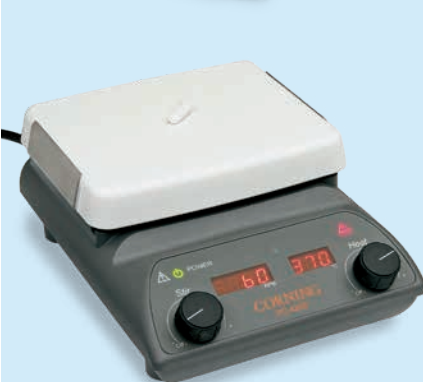
Corning® Stirring Hot Plates Closed-loop stirring control monitors and regulates stirring speed from 60-1,150 rpm for aqueous, viscous, or semi-solid solutions. Stronger, larger magnet improves stir bar coupling. Automatic ramp up speed adjustment minimizes decoupling. SB42262 Digital, 5" x 7" — $600.00 SB50648 Analog, 4" x 5" — $575.00
