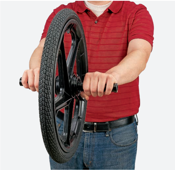
Bicycle Wheel Gyroscope Try to move the rubber wheel's axis of rotation. Suspend wheel from a string with aluminum handle. Hang weights from handle to investigate gyroscopic precession. 20" dia. SB21409 – $74.95
