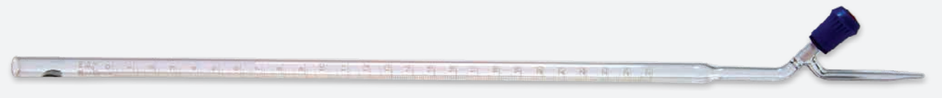
Glass Burette Borosilicate glass 50 ml burette. Individually calibrated. White enamel graduations. Graduation interval: 0.10 ml. General-purpose screw-thread stopcocks with PTFE keys provide excellent flow control and Fluon/glass seals that prevent leakage. SB39109 — $17.95
