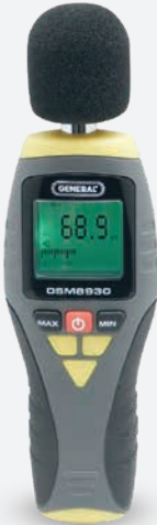
Digital Sound Meter Measure the loudness of equipment and vehicles or levels of environmental or industrial noise. Large backlit digital display, analog bar graph, and auto ranging. A-frequency-weighting and fast-time-weighting. Minimum/maximum memory with data hold, analog output, and auto power off after 20 minutes. Measurement range: 40–130 dB in 12 steps. Measurement accuracy: \pm 2.9'' \times 2\frac{1}{4}'' \times 1\frac{3}{4}'' . SB49326 – $89.95
