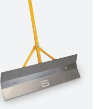
**HEAVY-DUTY FLOOR SCRAPER** Reversible blade. Angled handle allows for scraping even hard, frozen material. Handle and braces are triple-coated galvanized steel tubing. 7" x 24" blade; 58"L x 1" dia. handle. Stainless steel. 15-gauge steel. Allow extra delivery time. 🖡 C14590-\$79.99
