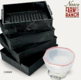
1/20" (1.27 mm) Sieve Only. Additional sieve containing smaller holes. Can be added to 3-Sieve Forage Particle Separator (C24682) with or without the  $\frac{5}{32}$ " sieve. Provides better characterization of smaller TMR feed particles for a more detailed measurement. C24078-\$139.99
