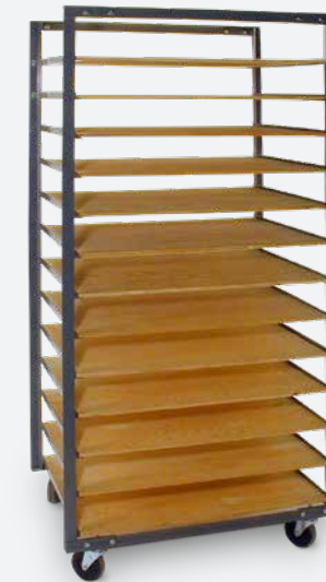
Bailey Ware Trucks Constructed of heavy-duty angle iron, vertical posts, and heavy gauge galvanized rungs. Each rack comes complete with 6" casters. The 13-division rack includes 13 pairs of rungs; the 26-division rack includes 26 pair of rungs that can be bolted in place at any spacing desired. Ideal for dinnerware or tile production. Shelves not included. Assembled dimensions: 34½"W x 24"D x 74¼"H. Assembly required. 13-Division Rack *Z15242 — $1,122.65 26-Division Rack *Z15243 — $1,544.95 Ware Boards. ½" AC plywood. 9719057 Half shelf, 12" x 32" — $22.90 *9719058 Full shelf, 24" x 32" — $46.30 *EXCLUDED FROM DISCOUNTS
