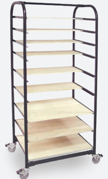
brent® Ware Cart EX Heavy-duty ware cart features top/bottom frame supports that bolt into place and powder-coated frame for durability and improved scratch and corrosion resistance. Side frames are 12-gauge steel with welded shelf supports. Square cross support tubes are 11-gauge steel. 35"W x 24"D x 72¾"H. The 4 heavy-duty, 4" rubber swivel casters roll easily when cart is loaded and can be firmly locked in place when needed. Comes with a set of 12" x 32", ½" thick exterior plywood shelves (shipped in a separate carton). Also includes plastic cover. Ware cart is shipped unassembled in 1 carton. Z08621 — $995.95
