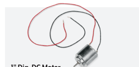
1" Dia. DC Motor Operates from 1.5V to 3V at .5V with no-load 80 to 90mA. .5 stall 200mA. Low torque; high rpm. 1" dia. x 1 1/2"L. 2 mm shaft. SB18068 — $4.95
