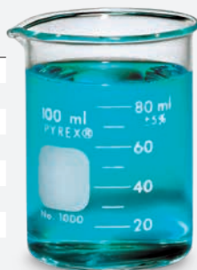
Corning® PYREX® Griffin Beakers – Low Form Uniform wall thickness. Optimum balance between thermal shock resistance and mechanical strength. Type I Class A per ASTM E438, E960 specifications. The 250–4,000 ml beakers have double-graduated metric scale.
