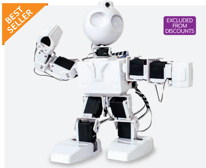
JD Humanoid Gr. 6–12 A fully functional humanoid robot kit featuring 16° of freedom and metal gear servo motors, meaning it has 16 motorized joints for walking, dancing, or anything you teach it. Eyes contain 18 RGB LEDs (9 per eye) that can be easily programmed and animated for unlimited expressions of up to 1 million colors. Compact grippers powered by strong, metal-gear servo motors for interacting with soft, light objects. A camera is contained in the robot’s head. SB52298 – $599.99
