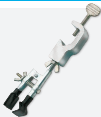
Burette Clamp — "V" Jaw Holds small objects. One jaw is flat; the other is "V" shaped with an opening of 3/16" to 1 3/8". Fits rods up to 3/4" (19 mm). Plastisol-coated jaws. SBI8968 — $6.95
