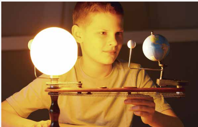
Trippensee® Hand-Driven Illuminated Planetarium Model Shows synchronized motions of Venus, Earth, moon, sun, and other planetary phenomena, including all the important Earth/moon/sun relationships. Light is used to illustrate lunar, solar, and annular eclipses; phases of the moon; and areas of day, night, and twilight. SBI5349 — $515.00
