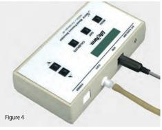
Pressure Simulator is ready for use. The unit has been factory calibrated for use with the accessories included in the kit. No further calibration adjustments should be necessary at this time. If the unit is to be used with a sphygmomanometer other than that supplied with the unit, or if recalibration is necessary at a later date, then see the section titled "Calibration Procedures".
