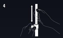
Loosen the screw to adjust the length.
