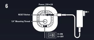
Insert the power plug into the back of Key Light Air, and the larger power brick into your nearest wall socket.
