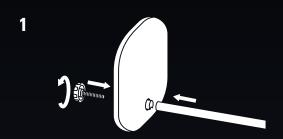
Secure the pole to the base using the included screw.
