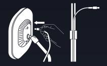
Connect the power supply and run the cable through the clip and rail.
