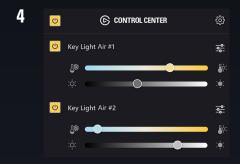
Use Control Center to switch Key Light Air on/off, adjust brightness, and finetune color temperature.
