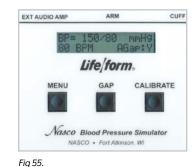
**Note:** The control box has a battery saving feature that will turn the unit off after approximately 8-10
