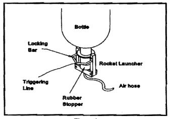
Figure 1 Attaching the rocket launcher to your bottle
