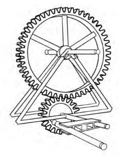
**Set-up two:** Crank on the lower axle. Put the yellow connector on the end of the upper axle where the blades used to be.
