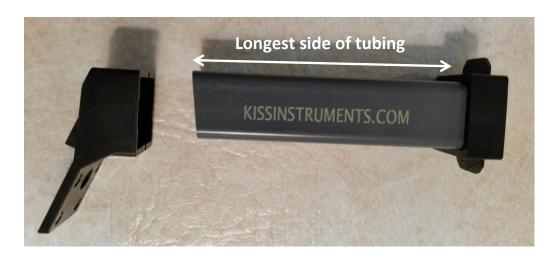
**3.** The slit is adjusted correctly. As illustrated, the slit needs to be adjusted to the correct side. Otherwise, you will not be able to calibrate the scope.
