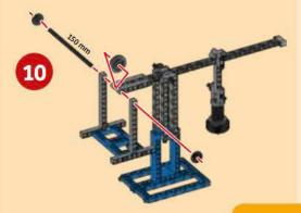
1 This balance scale is a class 1 lever. Try different loads in the basket and different locations of the weight on the other side.
